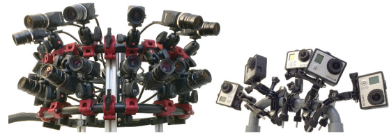
Figure 2: Two of the camera arrays we constructed for capturing the panoramic videos shown in this paper. Left: 14 machine vision cameras. Right: A small rig built using five GoPro cameras. Note that our panoramas have been captured without particularly accurate placement of cameras in order to demonstrate the flexibility of our approach.
