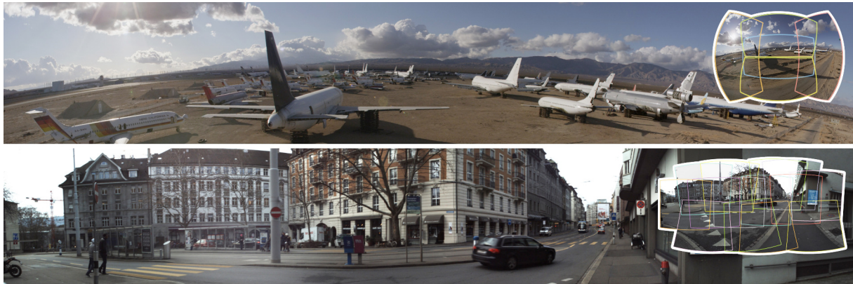
Figure 1: Two panoramas created with our system. Top - (00:05 in the accompanying video): a cropped frame from a 160 megapixel panoramic video generated from five input videos. The overlay on the right shows the full panorama, with the respective individual field of views of the input cameras highlighted by colored frames. Bottom - (01:22): a crop from a 20 megapixel panorama created from a highly unstructured array consisting of 14 cameras.
