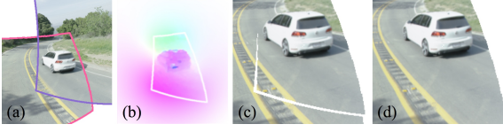
Figure 7: Importance of parallax extrapolation. (a) Two views aligned in the reference projection. (b) The interior of the white border visualizes the flow field (color encodes angle, saturation amplitude) computed on the overlap region for warping the bottom left image in (a) onto the top right image. Outside the white border the flow field has been smoothly extrapolated. (c) The warped result using only the interior of the overlap region. Note the tearing artifacts. (d) The warped result using the extrapolated flow in (b).
