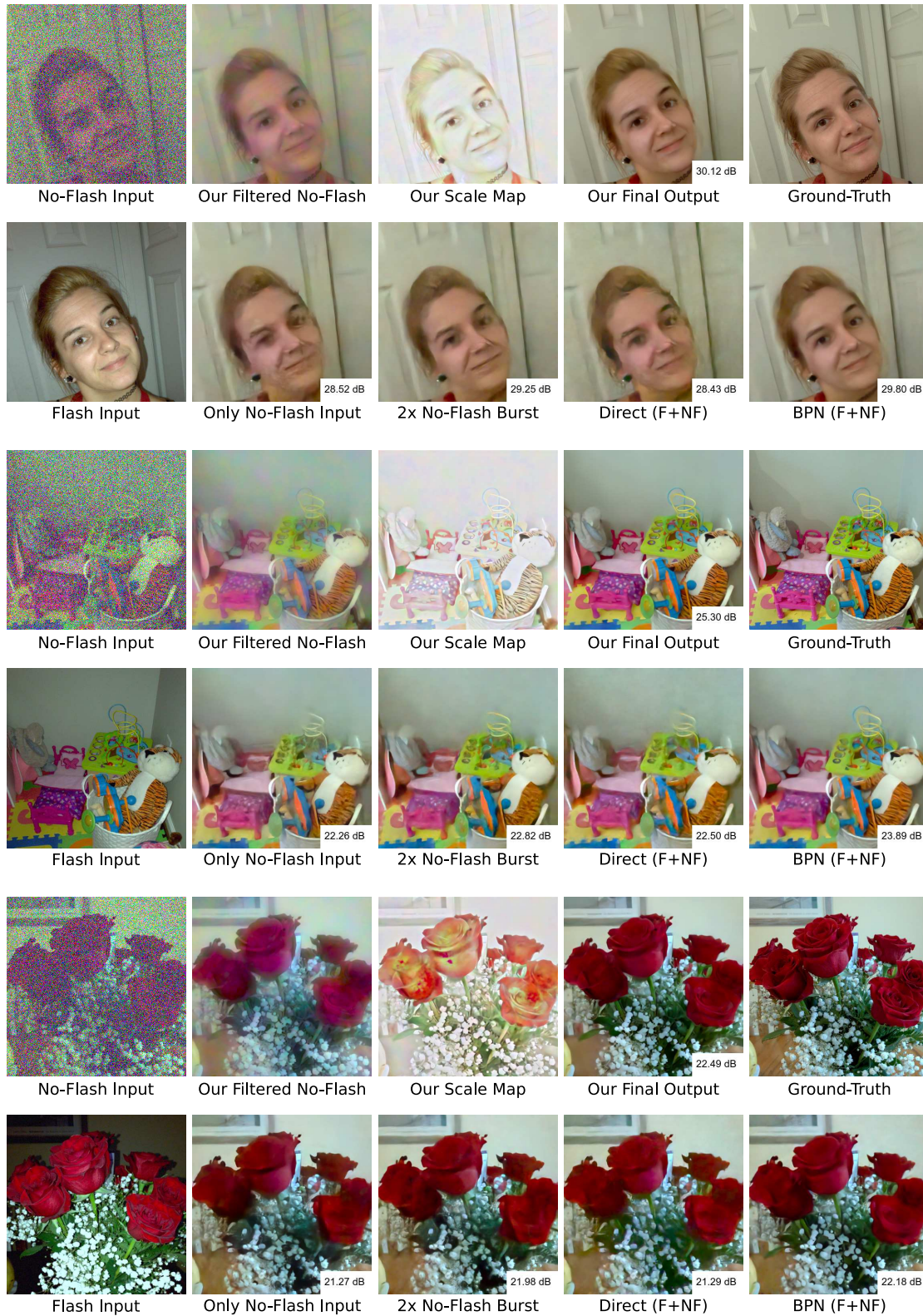
Figure 4: Qualitative comparison. Our method uses flash/no-flash image pairs to denoise low-light images. It produces cleaner outputs than baseline flash/no-flash denoisers ( Direct (F+NF) , BPN (F+NF) ), as well as single-image ( Only No-Flash Input ) and burst denoisers ( 2\times No-Flash Burst ). We also visualize our intermediate filtered no-flash image and scale map.
